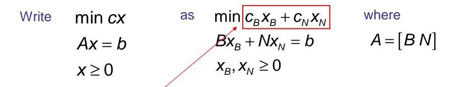
Solve constraint equation for  $x_B$ :  $x_B = B^{-1}b - B^{-1}Nx_N$
