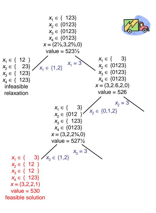
Solution is nonintegral, but we can backtrack because value of relaxation is no better than incumbent solution.
