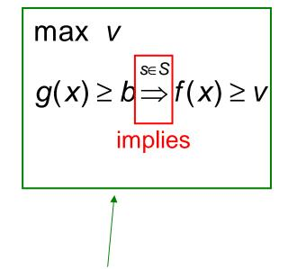
**Lagrangean Dual** problem: Find the tightest lower bound on the objective function that is implied by the constraints.
