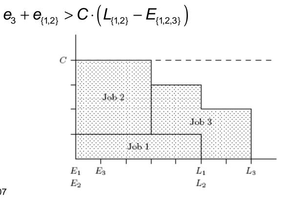
We can deduce that job 3 must finish after the others finish:  $3 > \{1,2\}$ Because the total **energy** required exceeds the area between the earliest release time and the later deadline of jobs 1,2:
