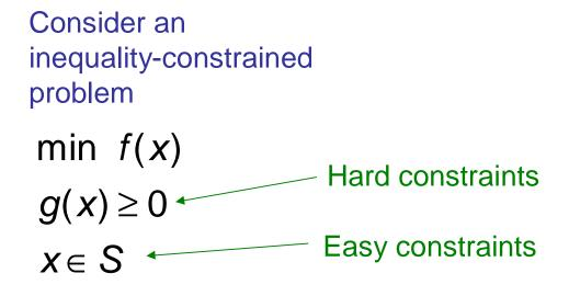
The object is to get rid of (**dualize**) the hard constraints by moving them into the objective function.
