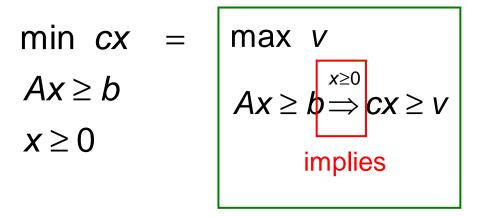
**Dual** problem: Find the tightest lower bound on the objective function that is implied by the constraints.
