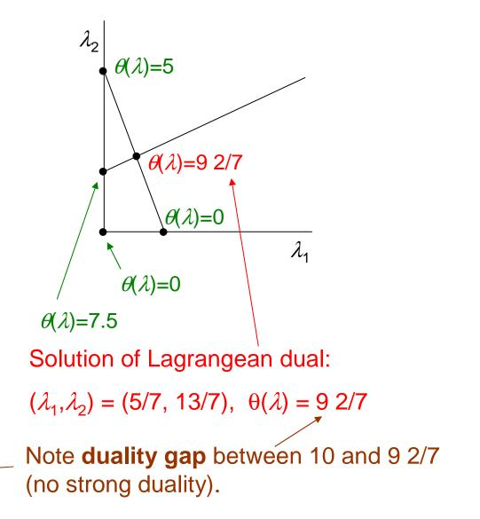
min  $3x_1 + 4x_2$  $-x_1 + 3x_2 \ge 0$  $2x_1 + x_2 - 5 \ge 0$  $x_1, x_2 \in \{0, 1, 2, 3\}$  Note: in this example, the Lagrangean dual provides the same bound (9 2/7) as the continuous relaxation of the IP.
