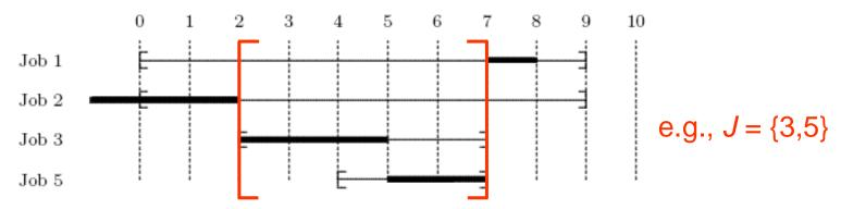
Removing a job from those within an interval only weakens the test  $L_{J \cup \{k\}} - E_J < p_{J \cup \{k\}}$
