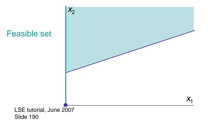
$$\begin{array}{ll} \min \ x_2 \\ x_2 \ge \begin{cases} 0 & \text{if } x_1 = 0 \\ f + C x_1 & \text{if } x_1 > 0 \end{cases} \\ x_1 \ge 0 \end{array}$$
