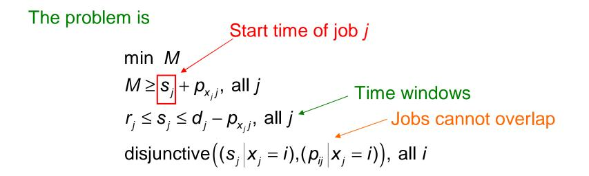
For a fixed assignment  $\overline{x}$  the subproblem on each machine *i* is
