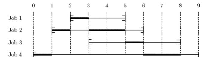
One  $O(n^2)$  algorithm is based on the Jackson pre-emptive schedule (JPS). Using a different example, the JPS is:
