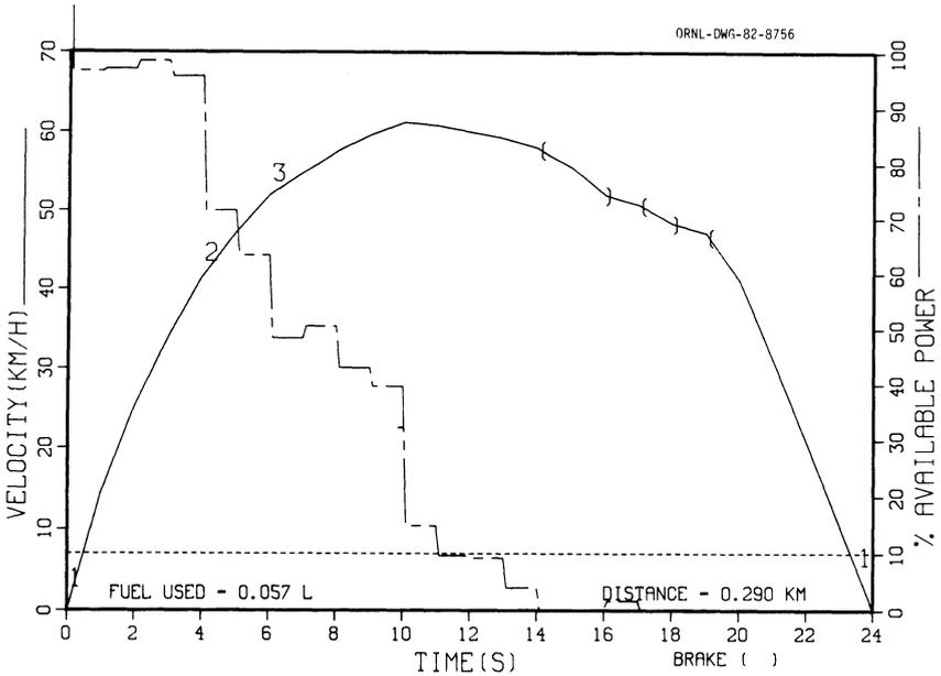
**Fig. 3.** Optimal control between stop signs on a 300-m block. The car is required to cover the distance in 24 s, and the maximum braking deceleration is 0.3 g.
