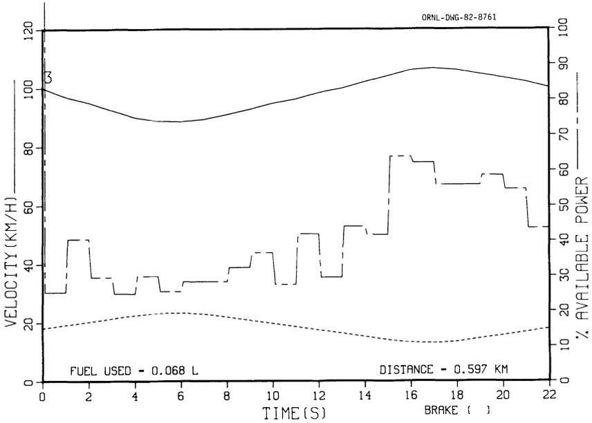
**Fig. 9.** Optimal control on a 0.6-km hill cycle with 6% grade. The initial, terminal, and average speeds are set at 100 km/h.
