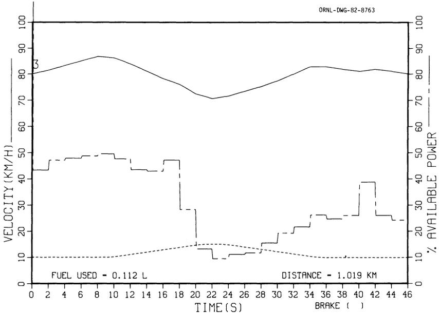
Fig. 11. Optimal control for driving over a 0.6-km isolated hill with 6% grade and 200 m of level road on either side.
