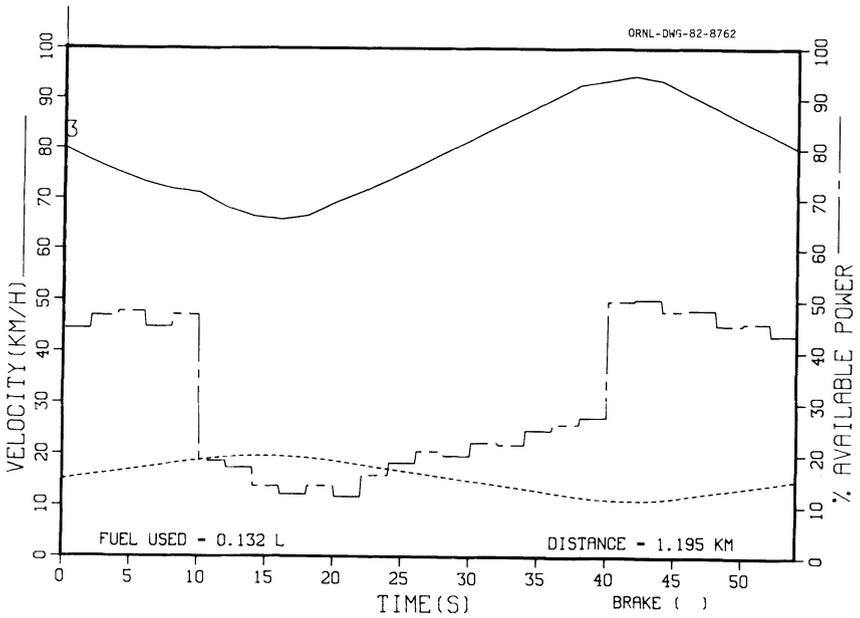
**Fig. 10.** Optimal control on a 1.2-km hill cycle with 6% grade. The initial, terminal, and average speeds are set at 80 km/h.
