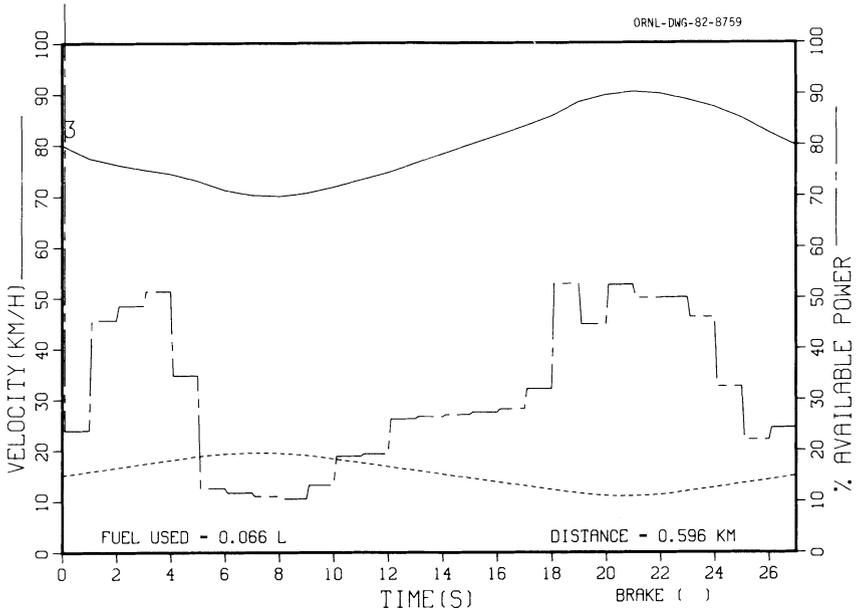
Fig. 7. Optimal control on a 0.6-km hill cycle with 6% grade. The initial, terminal, and average speeds are set at 80 km/h.
