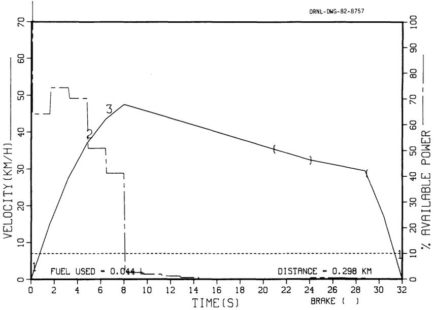
Fig. 5. Optimal control for a 32-s trip between stop signs on a 300-m block.
