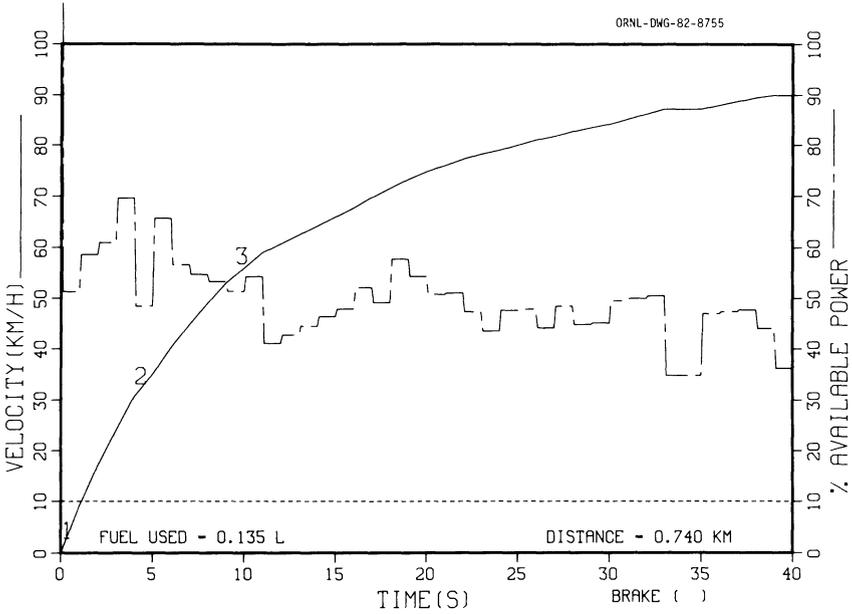
**Fig. 2.** Optimal acceleration from rest to a cruising speed of 90 km/h.
