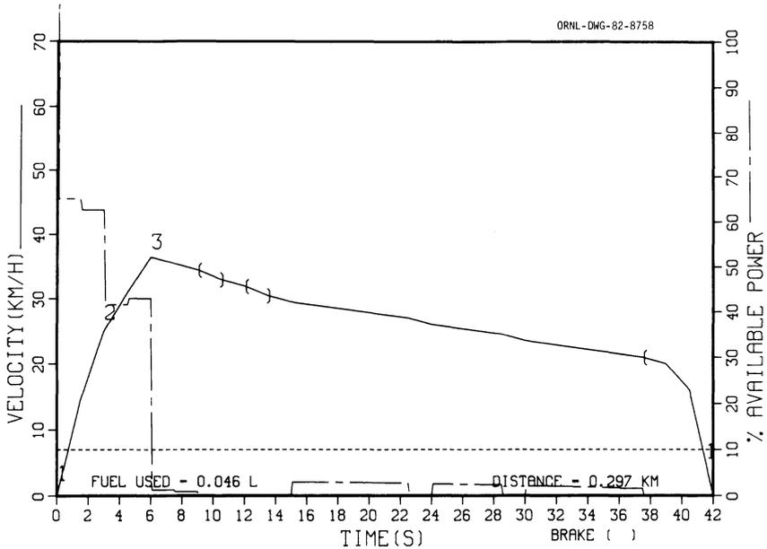
Fig. 6. Optimal control for a 42-s trip between stop signs on a 300-m block.
