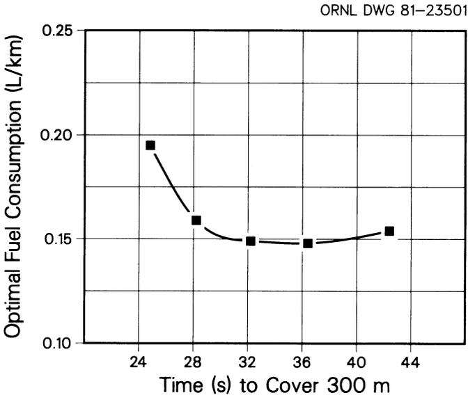
Fig. 4. Trade-off between time and fuel consumption for a 300-m block between stop signs.
