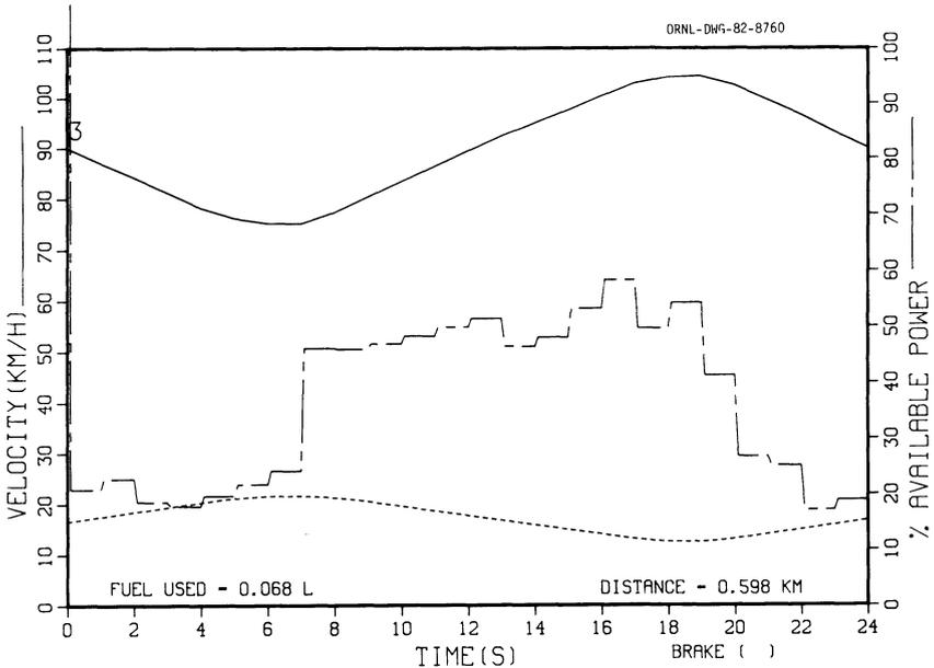
Fig. 8. Optimal control on a 0.6-km hill cycle with 6% grade. The initial, terminal, and average speeds are set at 90 km/h.
