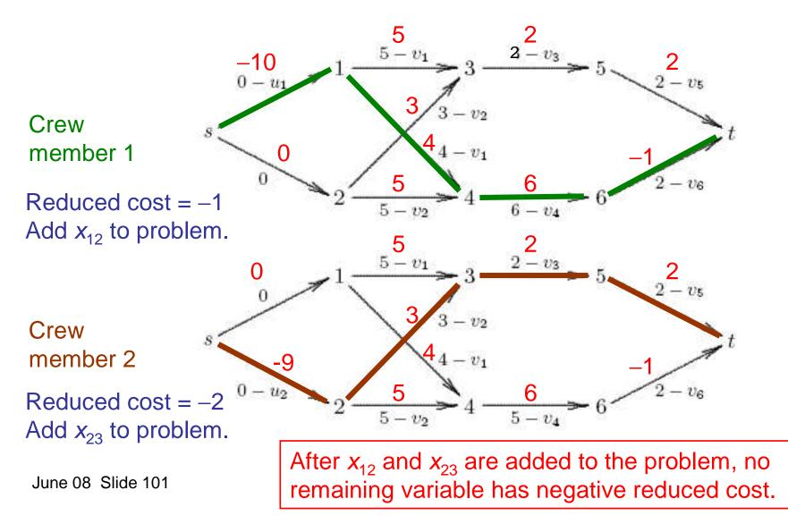
The shortest path problem cannot be solved by traditional shortest path algorithms, due to the bounds on total path length.
